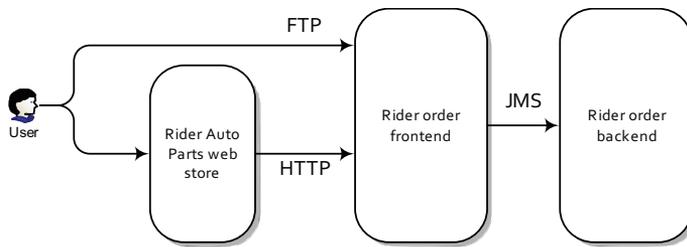
**Figure 2.2** A customer has two ways of submitting orders to the Rider Auto Parts order-handling system: either by uploading the raw order file to an FTP server or by submitting an order through the Rider Auto Parts web store. All orders are eventually sent via JMS for processing at Rider Auto Parts.
