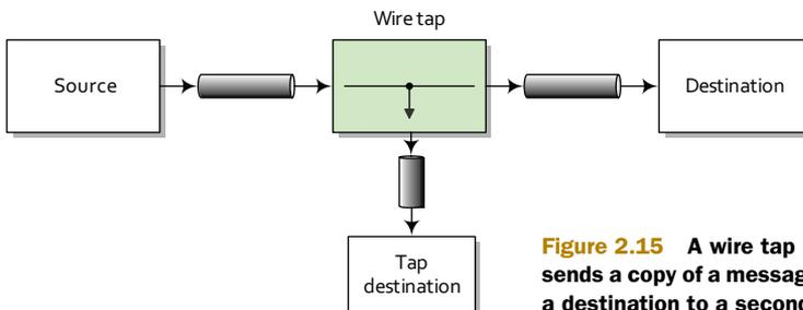
**Figure 2.15** A wire tap is a fixed recipient list that sends a copy of a message traveling from a source to a destination to a secondary destination.
