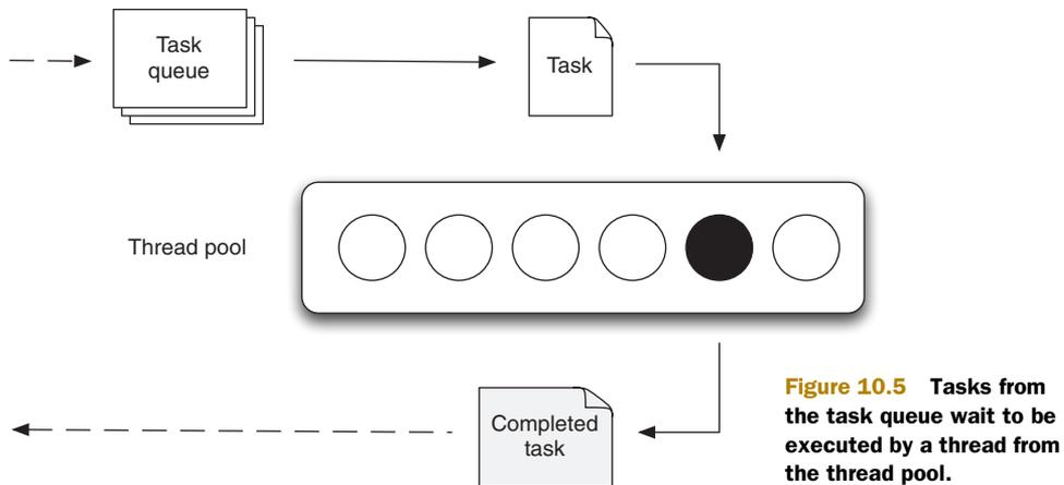
**Figure 10.5** Tasks from the task queue wait to be executed by a thread from the thread pool.
