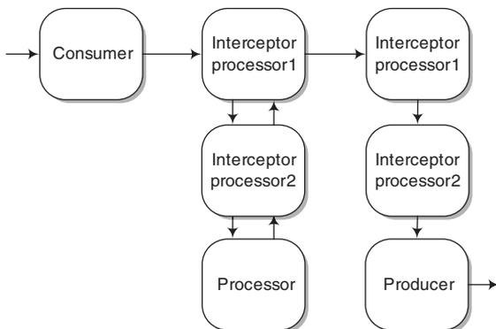
**Figure 11.10** Interceptors are stackable, meaning the more `InterceptStrategy` classes you add to the `CamelContext`, the more interceptor processors will be added before each real processor is executed.
