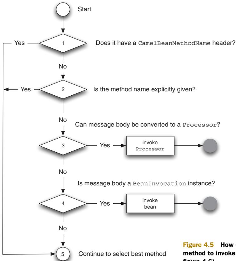
**Figure 4.5** How Camel selects which method to invoke (part 1, continued in figure 4.6)
