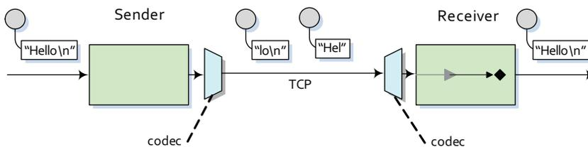
**Figure 7.11** During TCP communications, a payload may be broken up into multiple packets. A MINA `textline` codec can assemble the TCP packets into a full payload by appending text until it encounters a delimiter character.
