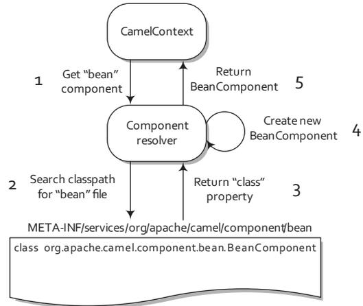
**Figure 7.2** To autodiscover a component named “bean”, the component resolver searches for a file named “bean” in a specific directory on the classpath. This file specifies that the component class that will be created is `BeanComponent`.
