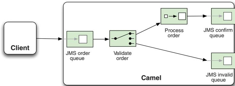
**Figure 6.5** The client sends orders to an order queue, which is routed by a Camel application. The order is either accepted and routed to a confirm queue, or it's not accepted and is routed to an invalid queue.
