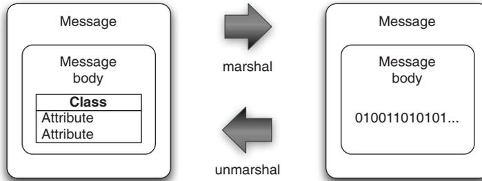
**Figure 3.6** An object is marshaled to a binary representation; `unmarshal` can be used to get the object back.
