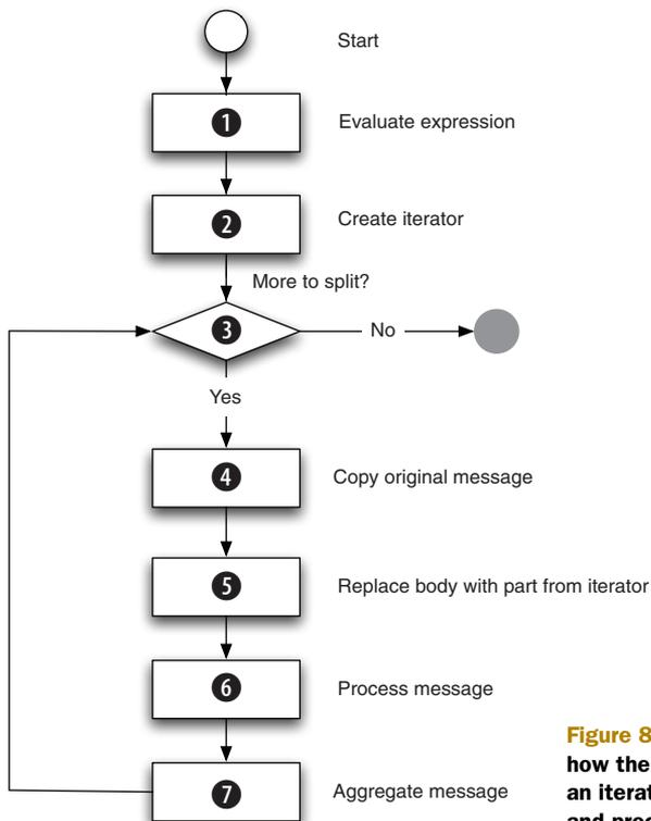
**Figure 8.7** A sequence diagram showing how the Splitter works internally, by using an iterator to iterate through the message and process each entry.
