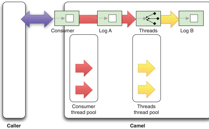
**Figure 10.11** In synchronous mode, the caller waits for a reply. On the Camel side, multiple threads are involved during the routing of the message. The consumer thread has to block, waiting for the reply, which it must send back to the waiting caller.
