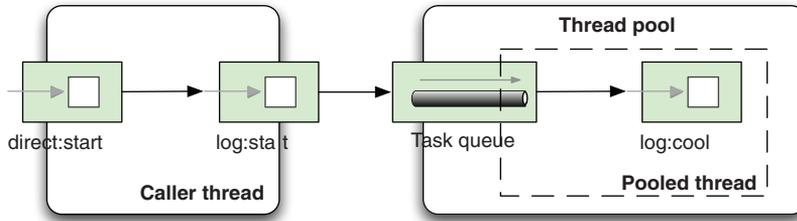
**Figure 10.6** Caller and pooled threads are in use when a message is routed.
