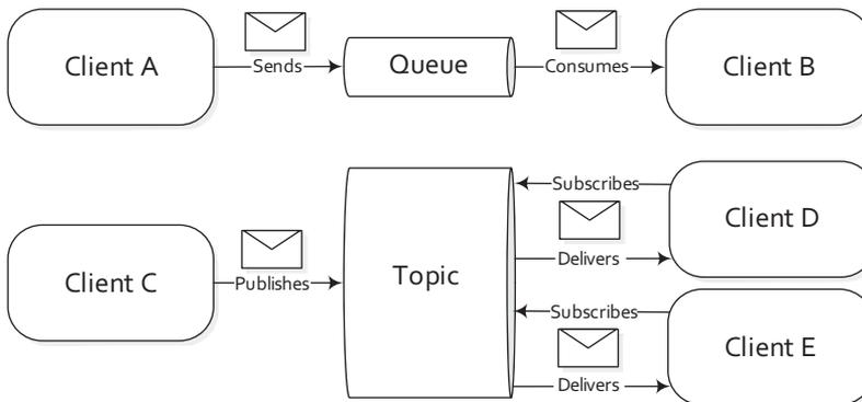
**Figure 2.4** There are two types of JMS destinations: queues and topics. The queue is a point-to-point channel, where each message has only one recipient. A topic delivers a copy of the message to all clients who have subscribed to receive it.
