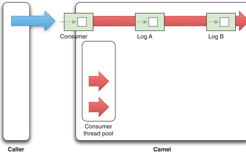
**Figure 10.8** In asynchronous `InOnly` mode, the caller doesn't wait for a reply. On the Camel side, only one thread is used for all the processing of the message.
