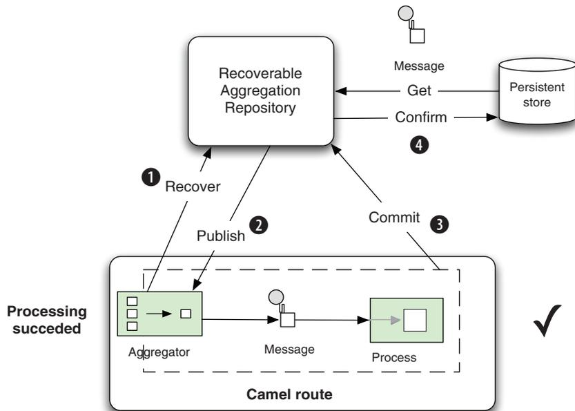
**Figure 8.5** The Aggregator recovers ❶ failed messages, which are published again ❷, and this time the messages completed ❸ successfully ❹.
