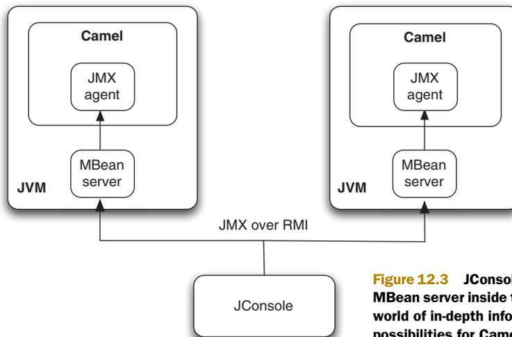
**Figure 12.3** JConsole connects remotely to an MBean server inside the JVM, which opens up a world of in-depth information and management possibilities for Camel instances.
