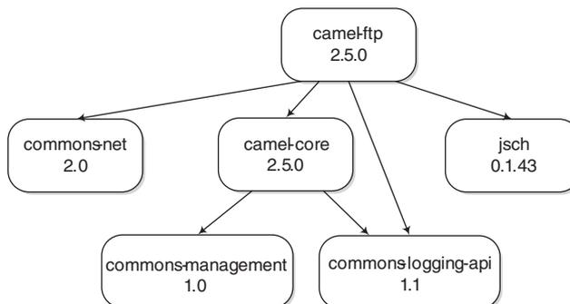
**Figure 11.2** Transitive runtime dependencies of the camel-ftp module. When you add a dependency on camel-ftp to your project, you'll also get its transitive dependencies added to your classpath. In this case, commons-net, camel-core, commons-logging-api, and jsch are added. Additionally, camel-core has a dependency on commons-management, so that's added to the classpath as well.
