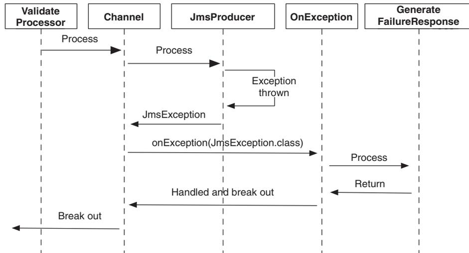
**Figure 5.5** Sequence diagram of a message being routed and a `JmsException` being thrown from the `JmsProducer`, which is handled by the `onException`. `onException` generates a failure that is to be returned to the caller.
