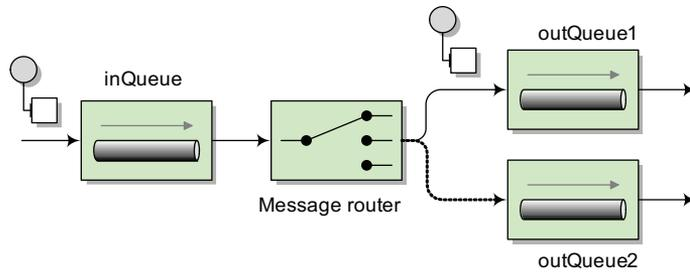
**Figure 2.1** A message router consumes messages from an input channel and, depending on a set of conditions, sends the message to one of a set of output channels.
