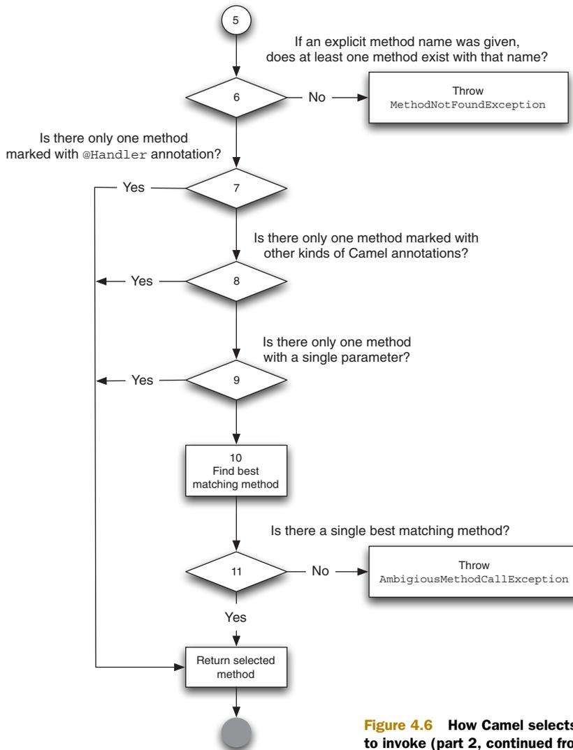
**Figure 4.6** How Camel selects which method to invoke (part 2, continued from figure 4.5)
