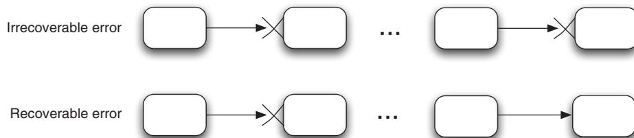
**Figure 5.1** Errors can be categorized as either recoverable or irrecoverable. Irrecoverable errors continue to be errors on subsequent attempts; recoverable errors may be quickly resolved on their own.
