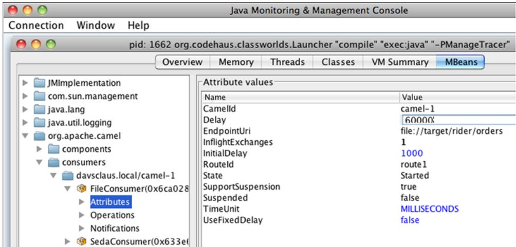
**Figure 12.11** Adjusting a file consumer at runtime by changing the Delay attribute
