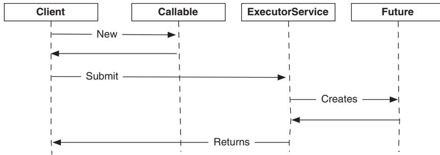
**Figure 10.13** The client submits tasks (Callable) to be executed asynchronously by ExecutorService, which returns a Future handle to the client.
