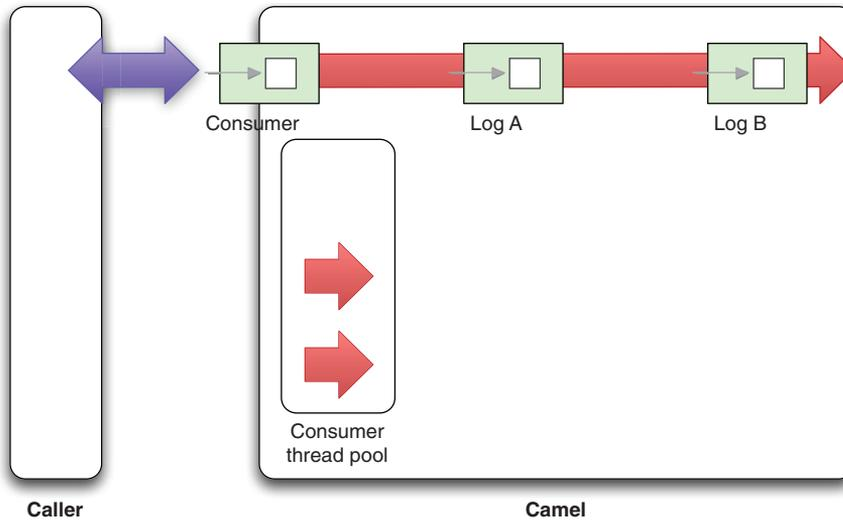
**Figure 10.9** In synchronous `InOut` mode, the caller waits for a reply. In Camel, the consumer thread is used for all the processing of the message, and it delivers the reply to the waiting caller.
