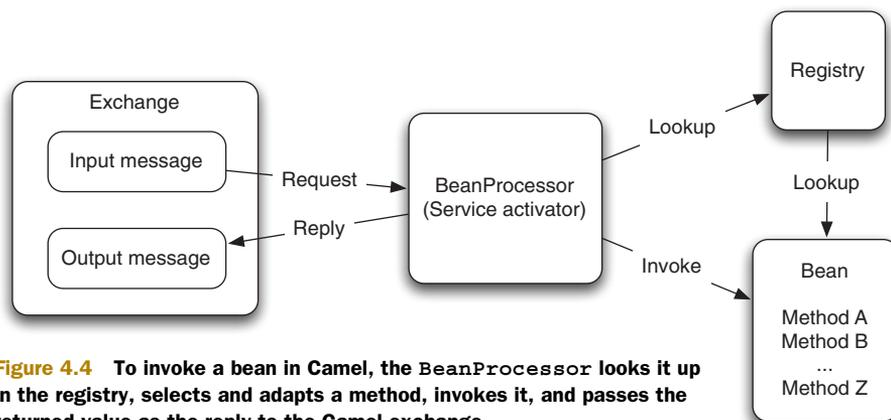
**Figure 4.4** To invoke a bean in Camel, the `BeanProcessor` looks it up in the registry, selects and adapts a method, invokes it, and passes the returned value as the reply to the Camel exchange.
