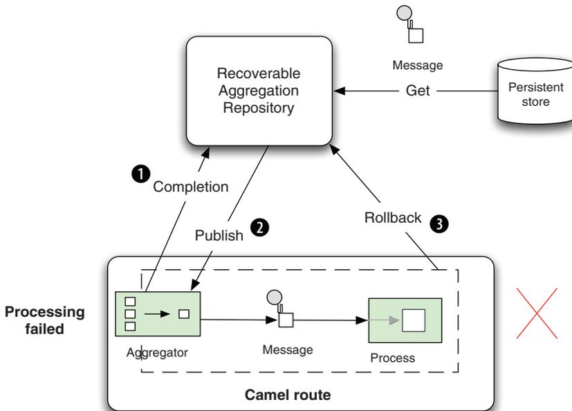
**Figure 8.4** An aggregated message is completed ❶, it's published from the Aggregator ❷, and processing fails ❸, so the message is rolled back.
