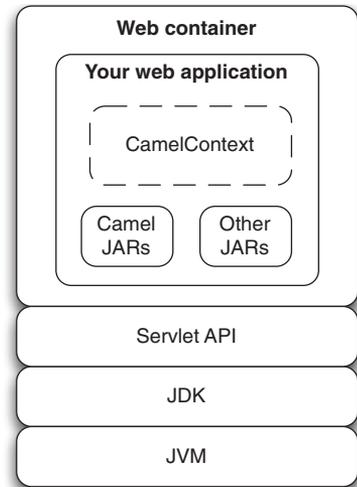
**Figure 13.7** Camel embedded in a web application
