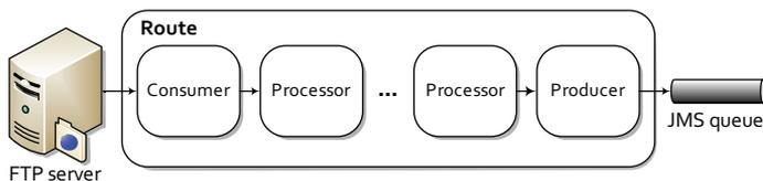
**Figure 11.8** A simplified view of a route where the consumer and producer handle interfacing with external systems. Consumers take messages from an external system into Camel, and producers send messages to external systems.
