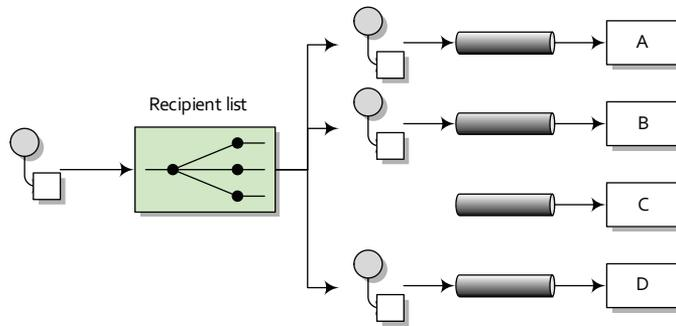
**Figure 2.14** A recipient list inspects the incoming message and determines a list of recipients based on the content of the message. In this case, the message is only sent to the A, B, and D destinations.
