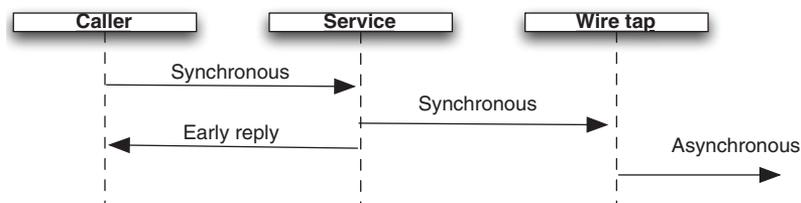
**Figure 10.12** A synchronous caller invokes a Camel service. The service lets the wire tap continue processing the message asynchronously while the service returns an early reply to the waiting caller.
