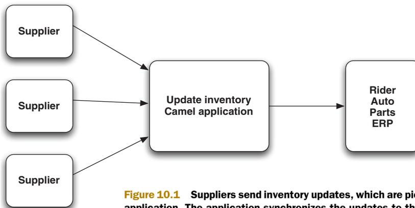
**Figure 10.1** Suppliers send inventory updates, which are picked up by a Camel application. The application synchronizes the updates to the ERP system.
