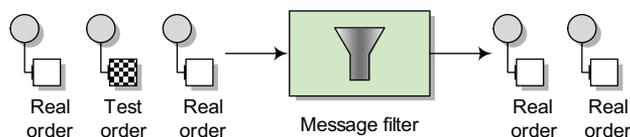
**Figure 2.12** A Message Filter allows you to filter out uninteresting messages based on some condition. In this case, test messages are filtered out.
