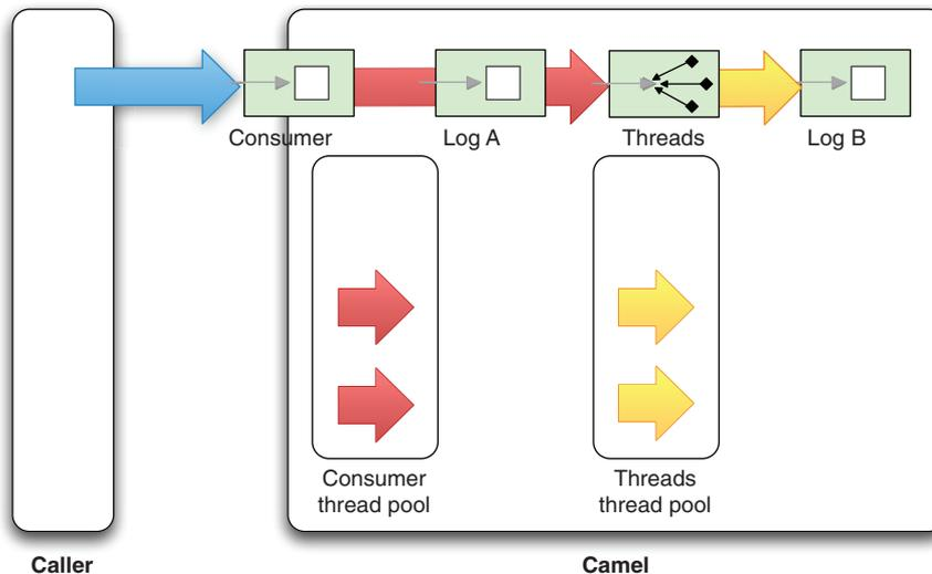
**Figure 10.10** In asynchronous InOnly mode, the caller doesn't wait for a reply. On the Camel side, multiple threads are involved during the routing of the message.
