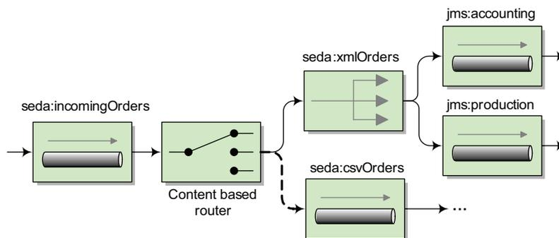
**Figure 7.14** SEDA queues can be used as a low-overhead replacement for JMS when messaging is within a CamelContext. For messages being sent to other hosts, JMS can be used. In this case, all order routing is done via SEDA until the order needs to go to the accounting and production departments.
