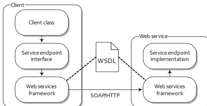
**Figure 7.7** A client invokes a remote web service over HTTP. To the client, it looks as if it's calling a Java method on the service endpoint interface (SEI). Under the hood, this method invocation passes through the web services framework, across a network, and finally calls into the service endpoint implementation on the remote server.
