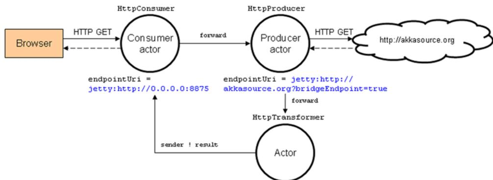
**Figure E.1** The setup of the example application. A consumer and a producer actor provide connectivity to external systems. The consumer actor receives requests from a browser and forwards them to a producer actor, which fetches the HTML page. The HTML page is then forwarded to an actor that transforms the content of the page and returns the transformation result to the initial sender, so that it can be displayed in the browser.
