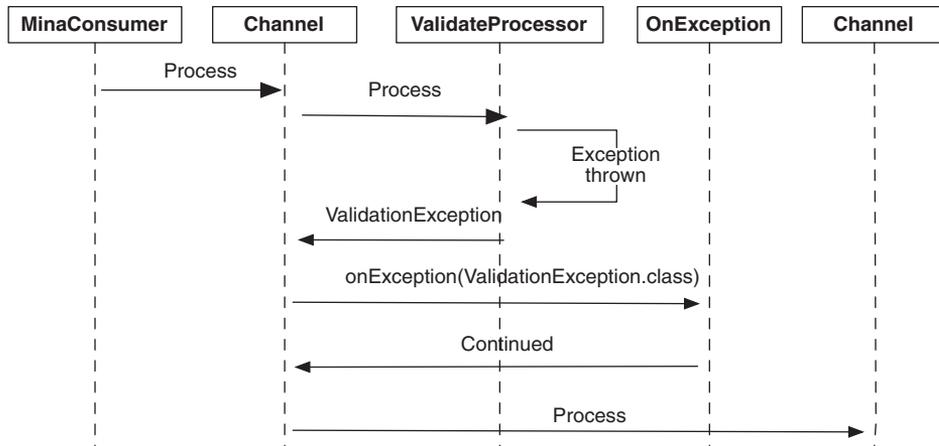
**Figure 5.6** Sequence diagram of a message being routed and a `ValidationException` being thrown from the `ValidateProcessor`. The exception is handled and continued by the `onException` policy, causing the message to continue being routed as if the exception were not thrown.
