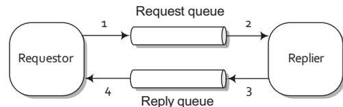
**Figure 7.5** In request-reply messaging, a requestor sends a message to a request queue and then waits for a reply in the reply queue. The replier waits for a new message in the request queue, inspects the `JMSReplyTo` address, and then sends a reply back to that destination.
