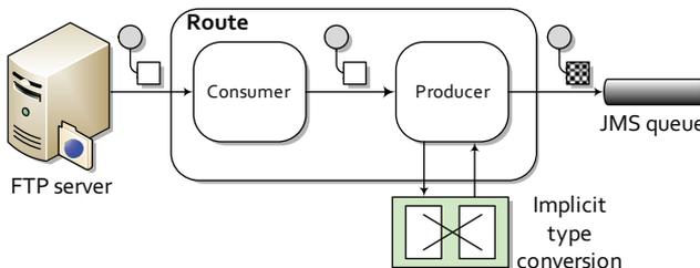
**Figure 2.8** The route shown in listing 2.1 forms a simple pipeline. The output of the FTP consumer is fed into the input of the JMS producer. The payload conversion from file to JMS message is done automatically.
