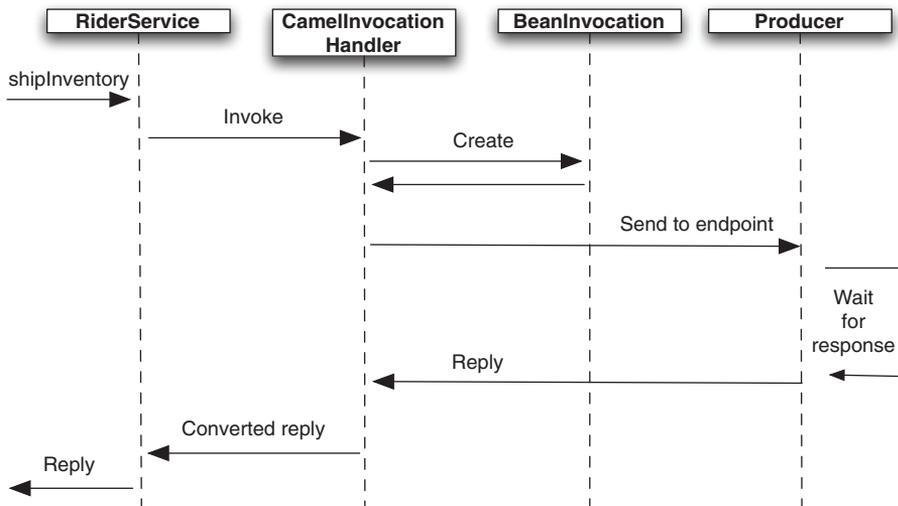
**Figure 14.5** A sequence diagram showing how a Camel proxy works under the covers, sending a `BeanInvocation` message to a remote endpoint and waiting for the reply, which eventually is returned to the caller
