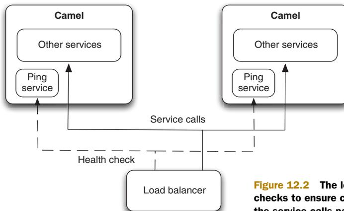
**Figure 12.2** The load balancer uses health checks to ensure connectivity before it lets the service calls pass through.
