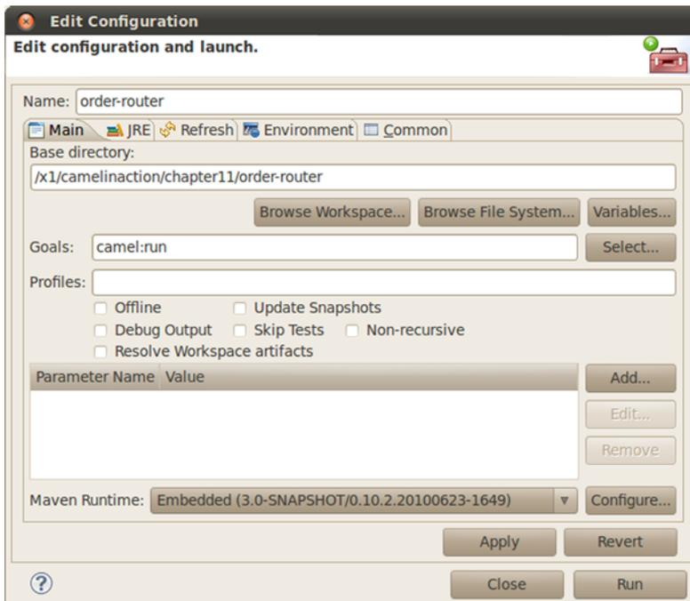
**Figure 11.6** Right-clicking on the order-router project in the Package Explorer and clicking Run As > Maven Build will bring up the Edit Configuration dialog box shown here. The `camel:run` Maven goal has been entered.
