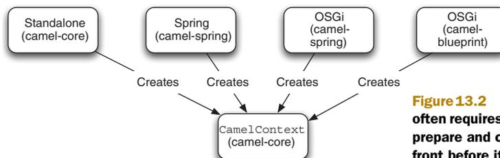
**Figure 13.2** Using Camel with containers often requires the container in question to prepare and create `CamelContext` up front before it can be started.
