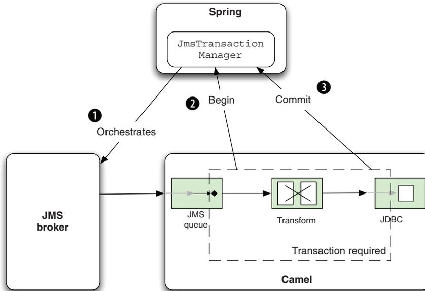
**Figure 9.4** The Spring `JmsTransactionManager` orchestrates the transaction with the JMS broker. The Camel route completes successfully and signals the commit to the `JmsTransactionManager`.
