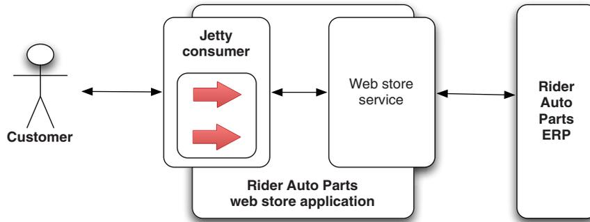
**Figure 10.14** The Rider Auto Parts web store communicates with the ERP system to gather pricing information.
