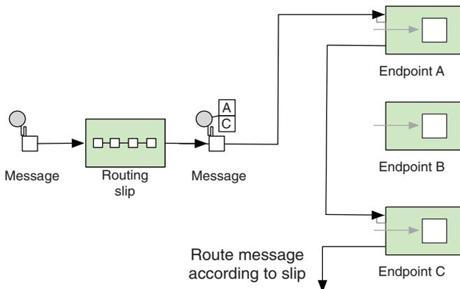
**Figure 8.11** The incoming message has a slip attached that specifies the sequence of the processing steps. The `Routing Slip` EIP reads the slip and routes the message to the next endpoint in the list.
