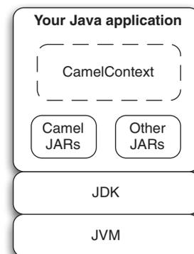
**Figure 13.6** Camel embedded in a standalone Java application
