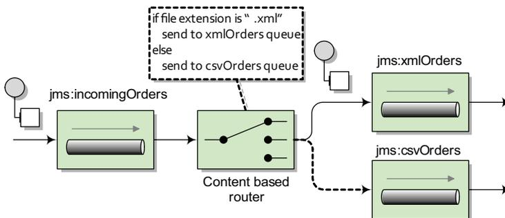
**Figure 2.10** The CBR routes messages based on their content. In this case, the filename extension (as a message header) is used to determine which queue to route to.
