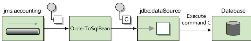
**Figure 7.13** A message from the JMS accounting queue is transformed into an SQL command message by the `OrderToSqlBean` bean. The JDBC component then executes this command against its configured data source.
