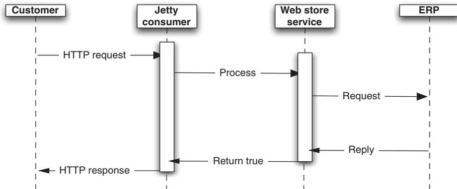
**Figure 10.15** A scalability problem illustrated by the thread being blocked (represented as white boxes) while waiting for the ERP system to return a the reply.
