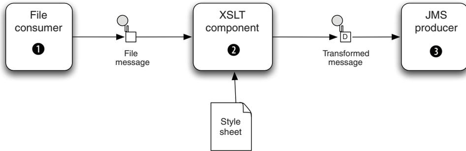
**Figure 3.5** A Camel route using an XSLT component to transform an XML document before it's sent to a JMS queue
